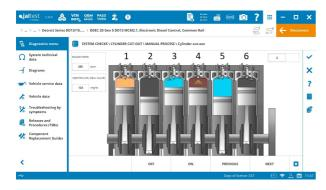
Extended coverage in all **DETROIT DIESEL-MBE** systems especially for 2023/2024 vehicles with new references and variants added. Furthermore, **DETROIT DIESEL-MBE** includes a new GIF System Display to simplify the cylinder cutout test interpretation.
